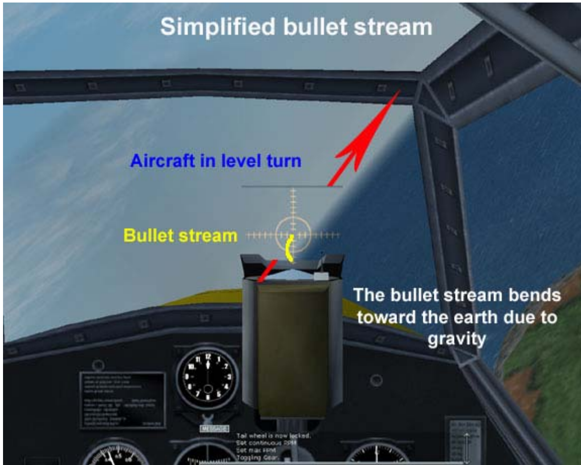
Figure 22 – Simplified bullet stream
