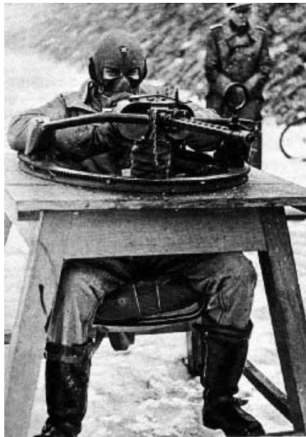
Figure 9 - MG 17 Ring and Bead sight
